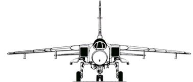
The shelter must be at least 0.5 metres above the top of the tail, and at least 1 metre clear horizontally of the wingtips.
